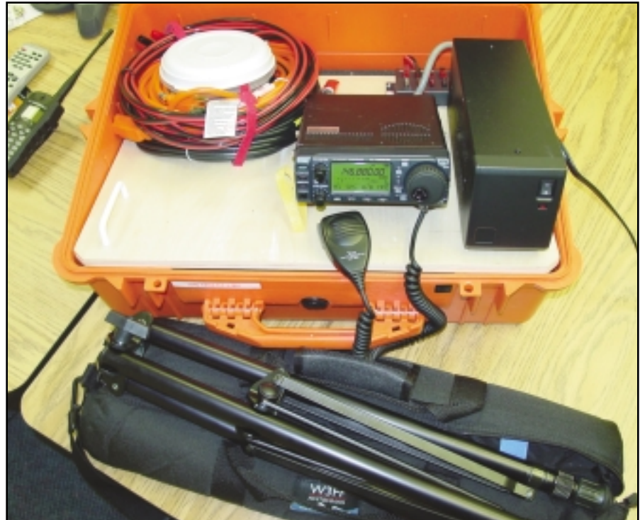
One of several HF radio go-kits shipped out to hospitals in Hawaii. (Photo courtesy of Toby Clairmont, KH7FR)
