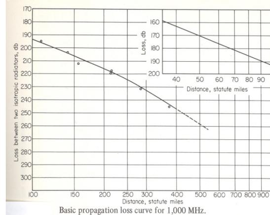
Fig.1: Tropospheric Propagation Loss between isotropic antennas at 1,000 MHz. (1) This loss in Fig. 1 includes the line of sight loss plus excess scattering loss. It assumes operation at 1.0 GHz with the antenna beams on the horizon. Simple but it is a big loss and there is more to come. One more chart to compensate for elevated antenna beams.
