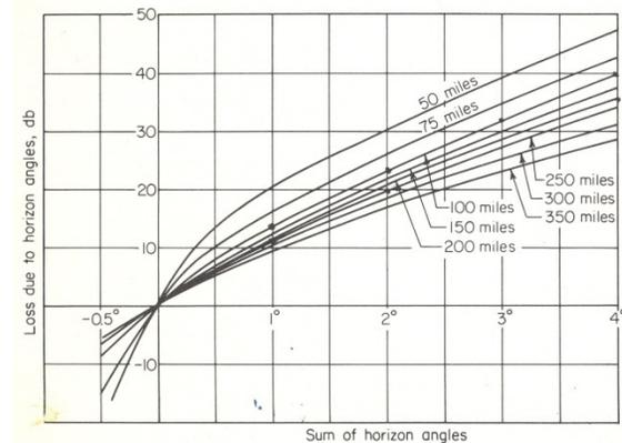
Fig. 2. Loss for elevated horizon angles. (1) The loss in figure 1 must be corrected for use at other frequencies. The frequency correction allows its use in the range of 100 to 4000 MHz. The correction in dB which is added to the loss from the chart is equation #1.
