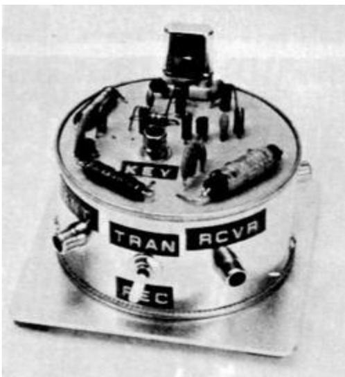
A May 1976 *QST* [article](#) by Doug DeMaw, W1CER, described how to build the Tuna-Tin 2 QRP transmitter for 40 meters.
